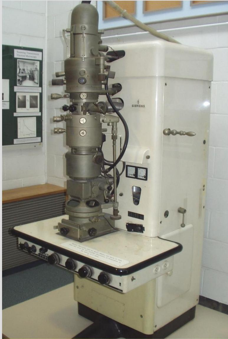
Electron Microscope used by Hirsch, Whelan, and Horne in 1956 when they made the first recorded observations of dislocations in the interior of a metal.
