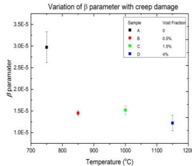
Figure 2. Variation in the  $\beta$  parameter of the samples as a result of creep damage.
