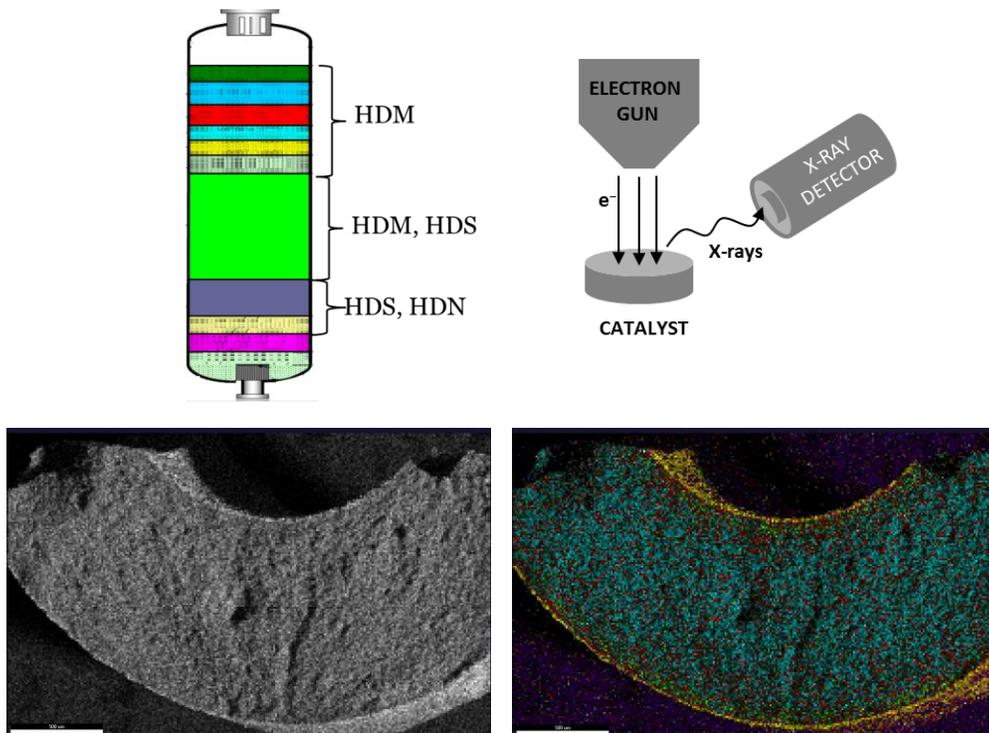
**Figure 1.** (TOP) Schematic representation of a Hydroprocessing reactor and the schematic of SEM-EDS. (BOTTOM) Cross sectional view of a typical HDM catalyst showing X-ray and false color elemental mapping.
