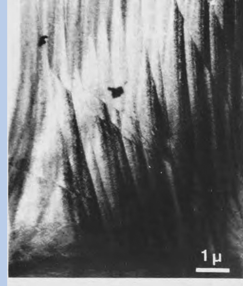
Fig. 1. 'Wave-like' pattern in MoO 3 film which should be regarded as the images of dislocations. (1954)
