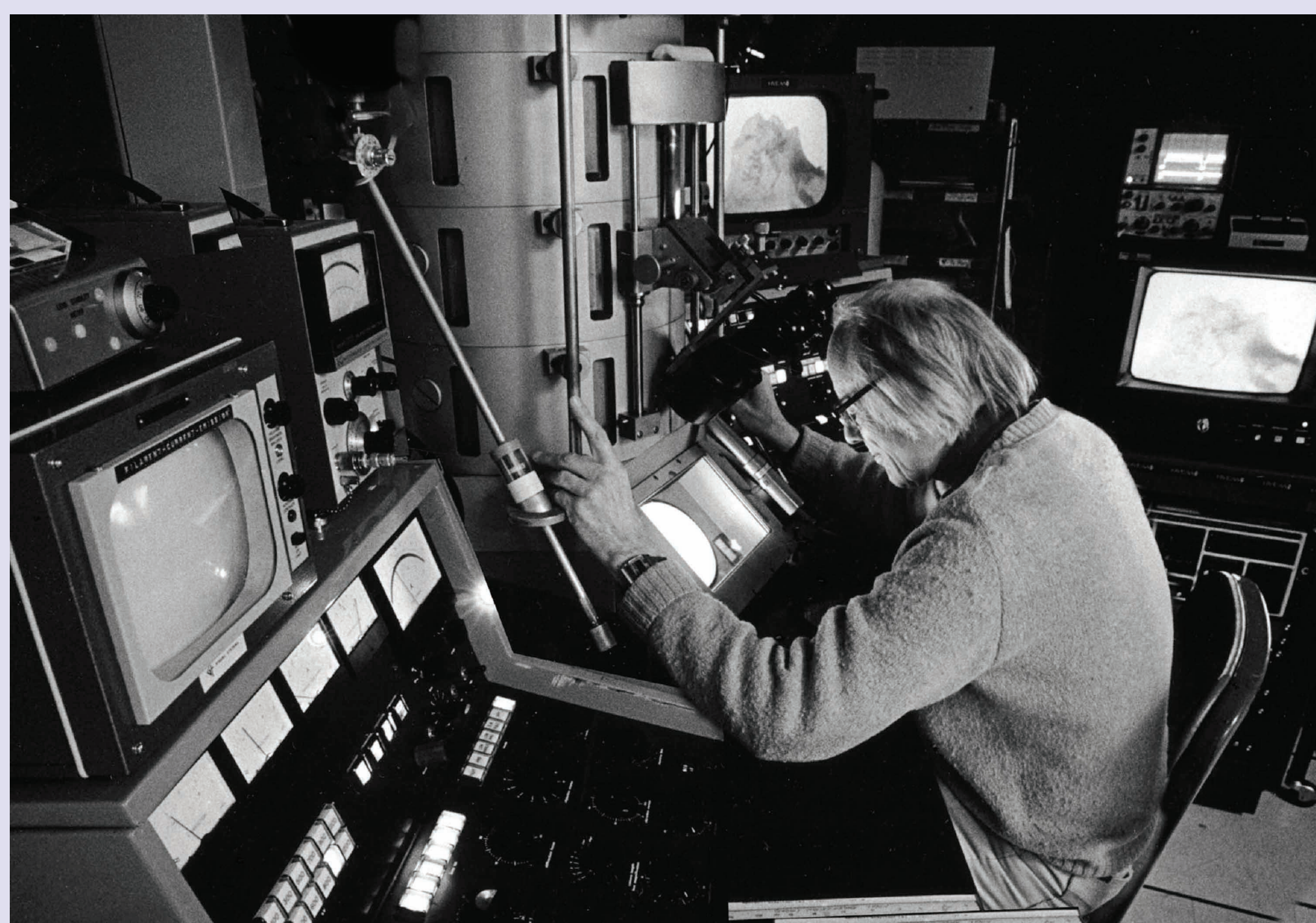
Hans Ris at the Madison AEI EM-7 million-volt electron microscope.
