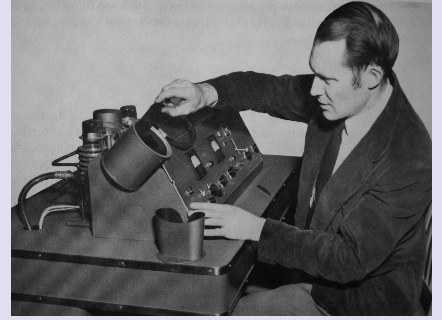
Fig. 2. Newberry operating his much-improved prototype GE electrostatic TEM, which was never marketed.
