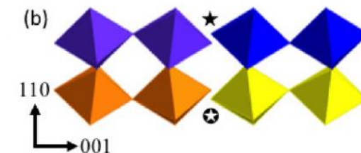
FIG. 6. Schematics of an APB in LSM ( R\bar{3}c ) viewed along different axes: (a) [110]_{pc} , (b) [1\bar{1}0]_{pc} , and (c) [001]_{pc} .
